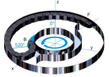
This type of horizontal arrangement allows rotation up to 520°. A customized guide channel is required.
